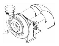
7. Adjust impeller, tighten clamp adapter set Mount hub cap. Mount V-belt protection
