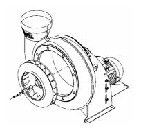
5. Fasten impeller with clamp adapter set on motor shaft (Do not tight yet the clamp adapter)
