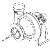
3. Fasten impeller with the clamp adapter set on motor shaft (do not tight yet the clamp adapter)
