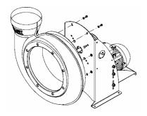
4. Attach casing to the support
