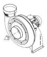
5. Adjust impeller, tighten clamp adapter set. Mount hub cap
