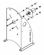
1. Install flanged bearings and support plates
