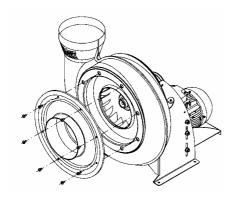
6. Fasten inlet section on the casing
