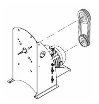
3. Install V-belt drive. Tension drive belt
