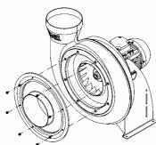
4. Fasten inlet section on the casing
